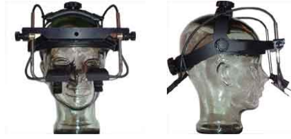
Figure 5.4: The Eyelink II eye head-mounted eye tracker uses corneal reflections to enhance its accuracy.
