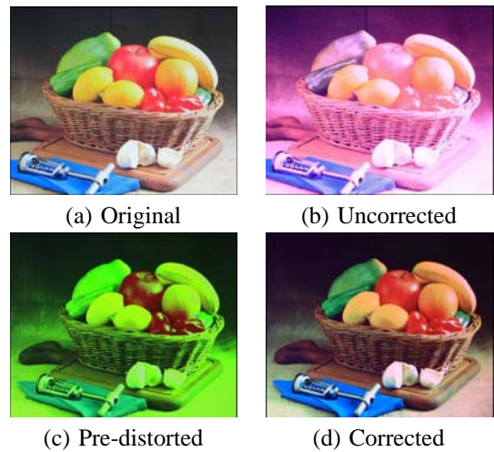
Fig. 4. Color correction results. (a) Original image (b) Original image displayed through a wavelength multiplexing filter, clearly showing an unnatural color shift. (c) Our algorithm pre-distorts the original image (d) After being displayed through the filter, the resulting image is close to the original. Note that all images were projected onto a white surface and photographed and so the camera imaging process had introduced additional color transformation and is only an approximation of what is actually observed by the human eye.
