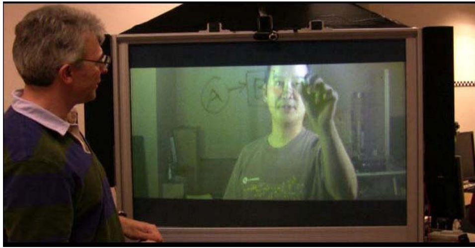
Fig. 6. ConnectBoard in action, linked to a second prototype in a remote location. Note that the image is horizontally flipped so that drawings made on the screen appear correct to both users.
