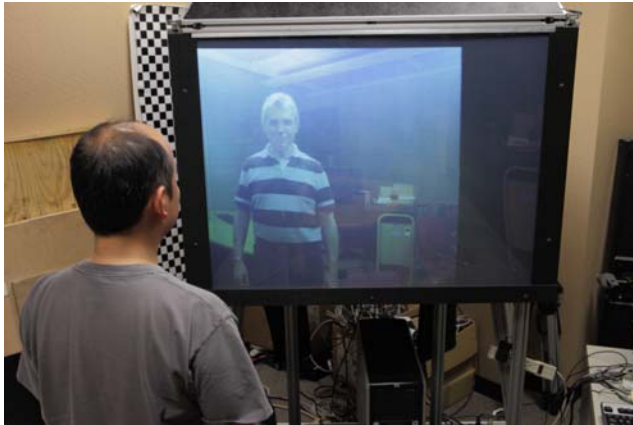
Fig. 11. Ensuring gaze awareness. As the remote user's image is shifted, the shared media (shown here digital composited) layer is also shifted correspondingly to ensure a correct rendering of the remote user's gaze direction with respect to shared content. At the same time, the users can make eye contact if they look at each other in the eye.
