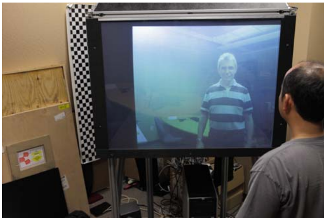
Fig. 10. Enabling eye contact. As the local user moves from the left side of the display to the right, the image of the remote user is automatically shifted so that the camera, local user's face, and remote user's face is always collinear. This way when the local user looks at the face of the remote user, he/she is always also looking into the camera, which captures the 'eye contact' view. The black bars in the screen in the top and bottom images serve to indicate the limits of the shared area between the two users. This subtly encourages local and remote users to position themselves such that the shared area is as large as possible, as is the case in the middle image.
