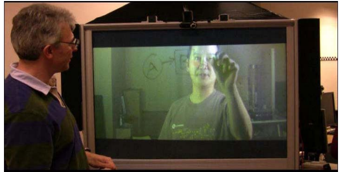
Fig. 1. ConnectBoard in action, linked to a second prototype in a remote location. Note that the image of the remote user is horizontally flipped so that drawings made on the screen appear correct to both users.
