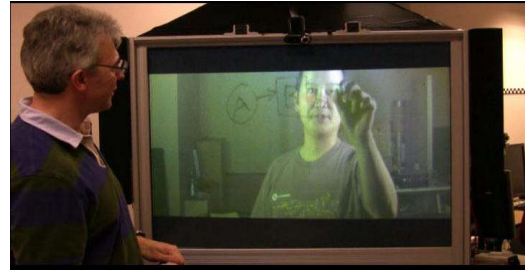
Figure 1. Two users collaborating on a ConnectBoard prototype with support for eye contact and gaze awareness.
