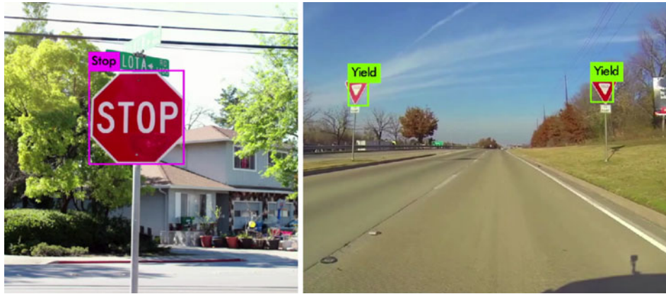
Fig. 13. Object detection with convolutional neural networks. A network trained to detect and recognize traffic signs may have applications in autonomous driving.
